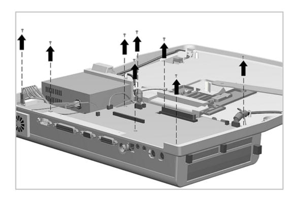
Figure 7-19. Removing the Main Board Screws
